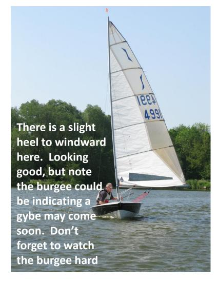
Overdoing the heel to windward can make the boat very unstable in a gust (remarkably he recovered from this)!
